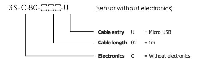
Order SS-C as spare sensors for the WE series measurement electronics
